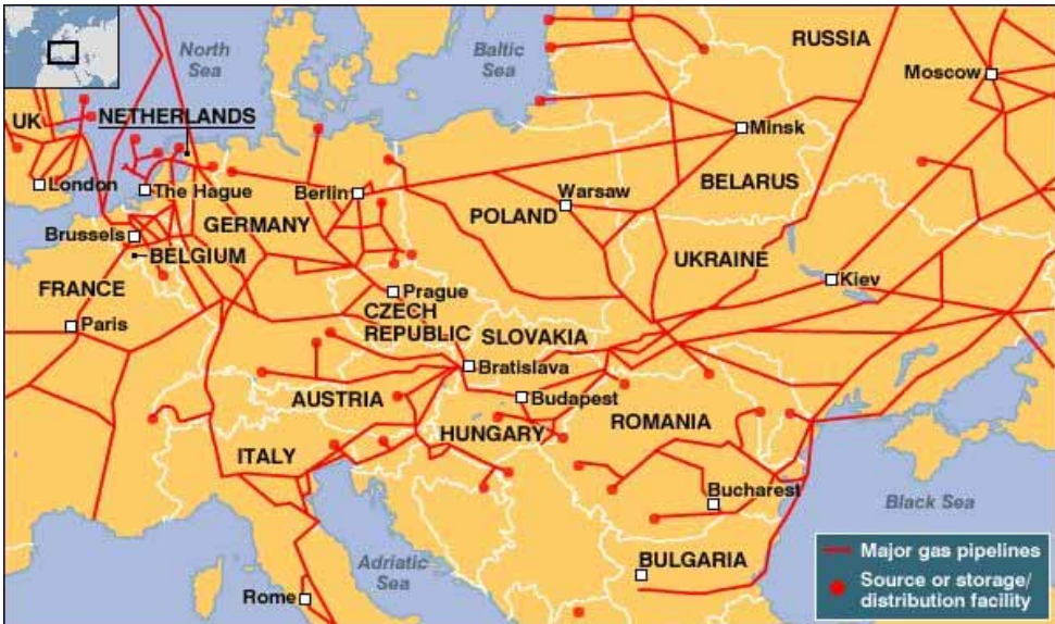
Figure A.3.1 Europe's gas pipeline network
